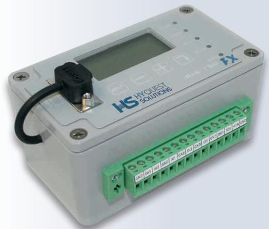
with laptops or other external equipment. A rubber cap provides protection when the port is not in use. The RS232 port operates in an auto-switching mode between terminal and binary modes at a default. A "telemetry" mode is provided where the port will revert to native iQuest protocol at a user-defined speed for telemetry applications.
